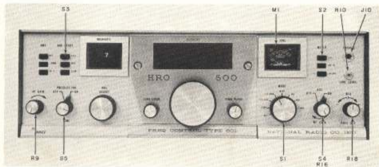
Figure 3-1. HRO-600 With Type 601 Plug-In Unit, Front View
